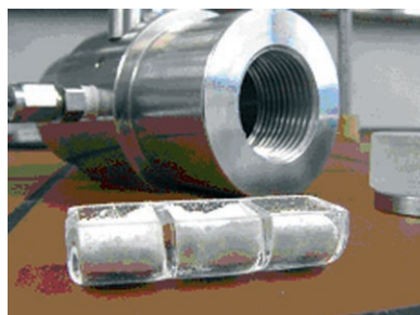
Figure 2. Experimental setup to show the simple compartmentalization for parallel hydroformylation reactions in \text{scCO}_2 .
